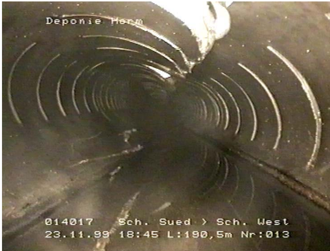
Figure 1: Damaged drainage pipe – axial crack
