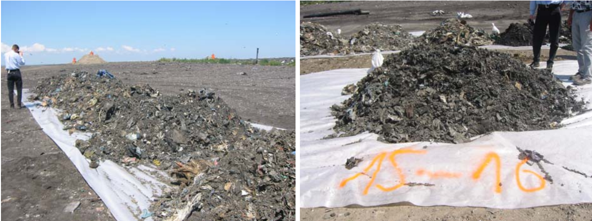
Fig. 15: Large drilling – exploited waste samples (one heap/2 m depth)
