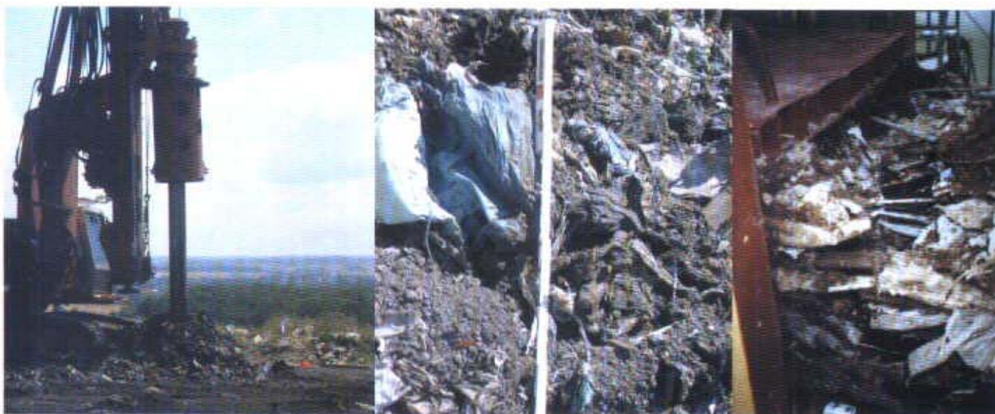
ABOVE LEFT AND CENTRE A sample being drilled at the Ihlenberg landfill for examination of waste composition and laboratory testing. ABOVE RIGHT The drilled sample undergoes a tension test under normal load, in which the internal angle of tensile stress, a material-specific value, is determined
